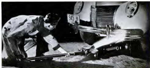
Pushing a button on the handle of the jack switches on the built-in spotlight
